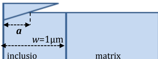
Fig. 1 Schematic of the indentation of two-phase biopolymer composites.
